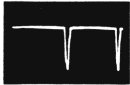
(W) Voltage Across Horizontal Deflection Coils of Yoke (L114, L115) (1440 Volts, P to P) (Pins 4 or 6 of V111 to Ground)
