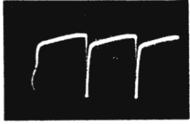
(T) Plate of Horizontal Discharge Tube (200 Volts, P to P) (Pin 5 of V108)
