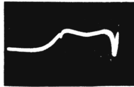
(X) Response of 1st and 2nd Video Amplifier Stages (Marker at 3MC on Left) (Video Sweep Input to Pin 1 of V105) (Output: Pin 2 of V113 Socket) (Diode Used Had 10 mmf. Capacity)
