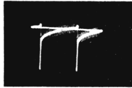
(N) Grid of Vertical Oscillator Tube (200 Volts, P to P) (Pin 1 of V107)
