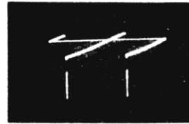
(O) Input to Vertical Output Tube (45 Volts, P to P) (Junction of C129 and C130)
